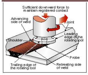
Fig. 1: Schematic diagram of the FSW process
