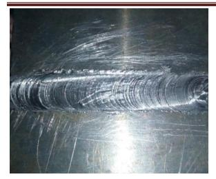
Fig. 3 Snapshot of AA plates welded at 1200 rpm
