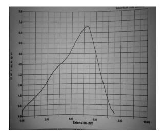
Fig. 5 Graph of Tensile Test (Load vs. Extension)
